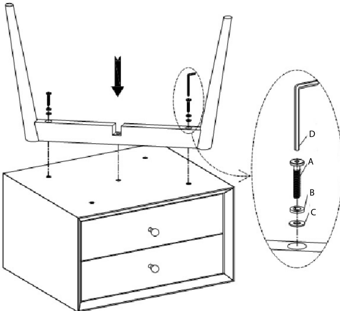
1. Align leg as shown. Insert bolt (A), lock washer (B), and flat washer (C). Tighten with supplied hex key (D).
