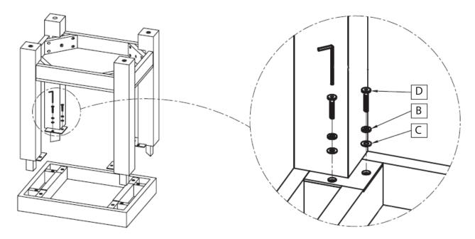
3. Tighten all bolts completely using supplied hex key. Turn assembled table upright.
