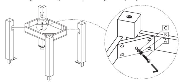
2. Lay top upside down on a clean smooth surface. Align assembled shelf and legs over top. Slide legs into the bottom of the top. Insert bolt (D), spring washer (B), and flat washer (C), into the holes shown. Tighten with supplied hex key.
