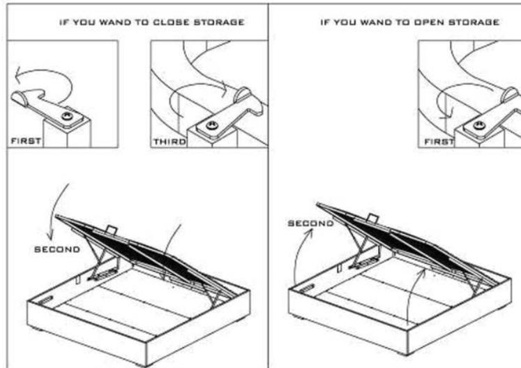
Make sure lock is engaged when mattress is not on metal frame to be sure that the metal frame does not raise unexpectedly.
