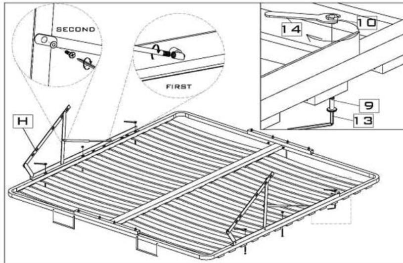
8. Turn the assembled metal slats frame upright with a helper and attach the hydraulic arms (H) to the side rails (C) with crosshead bolts (11), and flat washers (12). Tighten with phillips head screwdriver.
