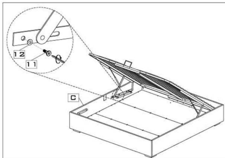
9. To close the storage bed, open the latches on the footboard and pull the metal slats frame down and lock latches as shown below. To open the storage bed, open the latches and pull metal slats frame up as shown below.
