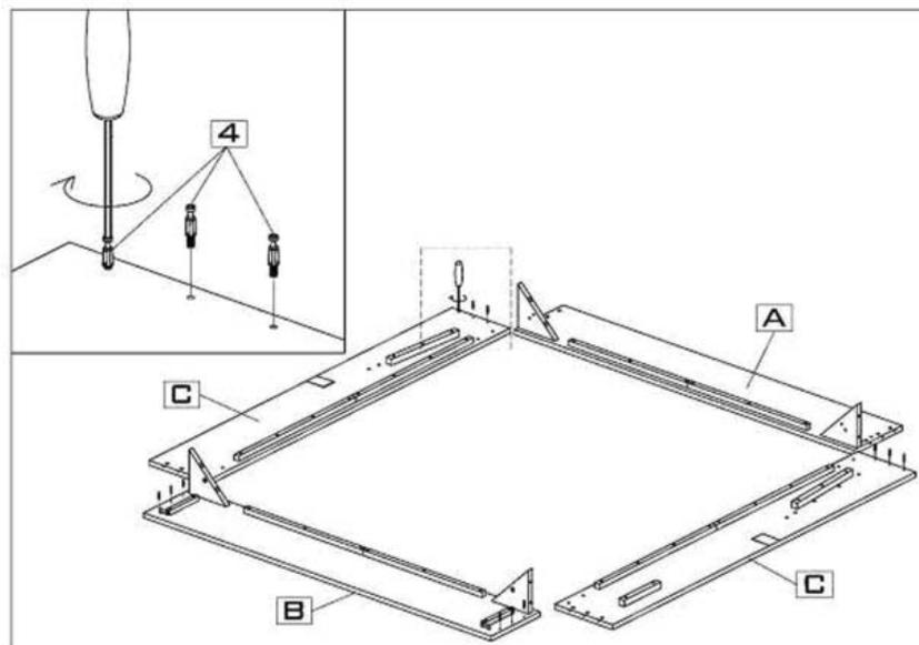
3. Attach the side rails (C) to the headboard (A) and the footboard (B) with bolts (1), spring washers (2), and flat washers (3). Tighten with allen key (8). Insert cam lock (5) into the headboard (A), and side rails (C). Tighten cam locks (5) with phillips head screwdriver as shown below.
