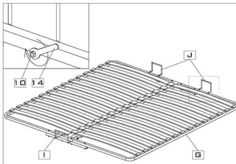
7. Turn the metal frame over and attach the two hydraulic arms (H) to the metal slats frame (G) with bolts (9), and hexagon-nuts (10). Tighten with allen key (13) and spanner wrench (14).
