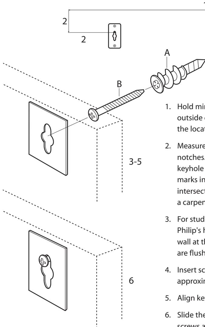
! For drywall mounting, use anchors with screws.
