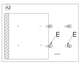
2. Use a Phillips Screwdriver to insert the Drywall Anchors (E) at the marked locations. Do not "push" or drive the Drywall Anchors (E) into the wall, it is designed to bore into the wall like a drill bit. Slowly turn the Drywall Anchors (E) clockwise while applying pressure until the flange just touches the wall.
