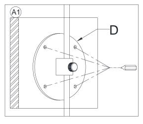
Place the Mounting Plate (D) against the wall at the desired mounting location. Using a pencil to make 4 insertion markings on the wall through the holes of the Mounting Plate (D).
