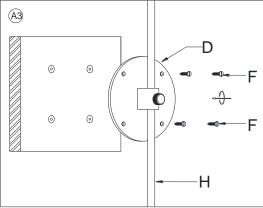
Attach the Mounting Plate (D) onto the wall aligning the 4 holes with the 4 pre-drilled pilot holes. Insert the 4 Mounting Screws (F) with a screwdriver and rotating clockwise to secure the Mounting Plate (D) in place.
