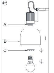
Attach the Shade (B) onto the Socket (A). Secure Shade
