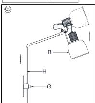
If needed, loosen the Clamping Nut (G) by turning anticlockwise.
