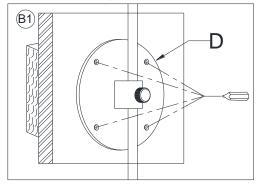
Place the Mounting Plate (D) against the wall at the desired mounting location. Using a pencil to make 4 insertion markings on the wall through the slots of the Mounting Plate (D).
