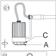
1. Unscrew the Socket Ring (C) from the Socket (A) by rotating counter-clockwise.
