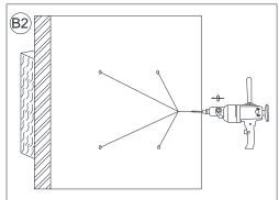
2. Pre-drill pilot holes at the marked locations. This will make installing the Mounting Screws (F) into the wall easier.
