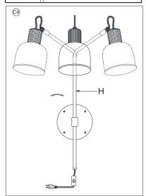
4. If needed, adjust the light fixture to your desired direction by rotating the Tube (H) to the left or right.
