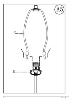
Raise the harp caps and insert the bottom ends of Harp (F) into the Saddle (D). Lower the harp caps until cover the two-pronged Saddle(D).
