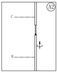
2. Screw the top end of Lower Tube (B) into Upper Tube (C) by turning clockwise until tight.
