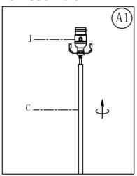
Screw Upper Tube (C) onto the bottom threaded end of Socket
