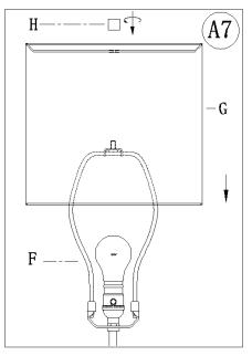
Place the Lamp Shade (G) over Harp (F). Making sure the harp top extends through the top ring of Shade (G). Secure the Shade (G) by turning the Final (H) onto the harp top until tight.
