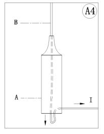
4. Gently pull the excess Cable (I) out from the Lamp Base (A) as shown and ensure cable is not twisted.
