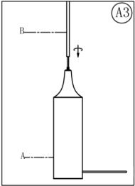
3. Attach the bottom end of Lower Tube (B) onto the threaded nipple of the Lamp Base (A) and turning clockwise until tight.
