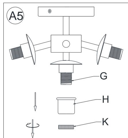
5. Unscrew the Socket Rings (K) and Spacers (H) from the Sockets (G) by rotating the Socket Rings (K) in a counter-clockwise direction.
