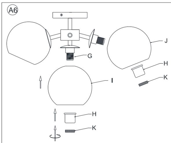
6. Attach the Large Glass Shade (I) onto the bottom Socket (G) and attach the four Small Glass Shades (J) onto the four side Sockets (G). Place the Spacers (H) onto the Sockets (G). Secure Glass Shades (I/J) and Spacers (H) by rotating the Socket Rings (K) in a clockwise direction until tight.
