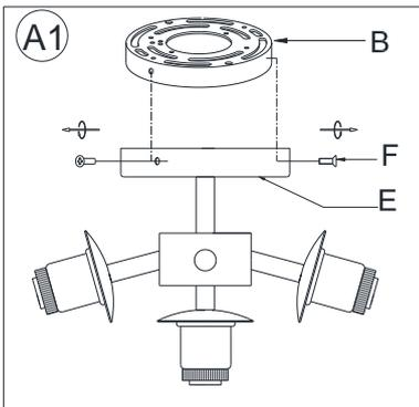
1. Separate the Mounting Plate (B) from the Canopy (E) by removing the 3 Canopy Screws (F). Do not discard the Canopy Screws (F) as these will be used later.
