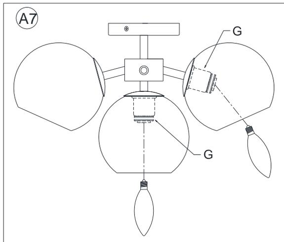
7. Insert the specified light bulbs into the Sockets (G). DO NOT EXCEED THE SPECIFIED WATTAGE.
