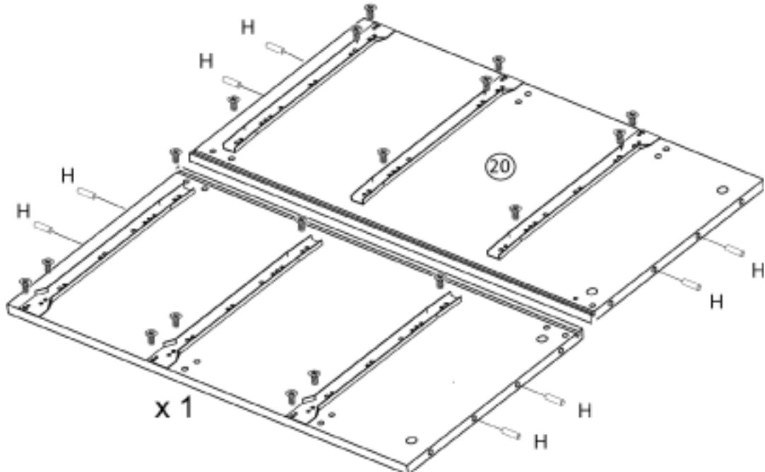
8. Insert 4 large wooden dowels (H) into the back rails.
