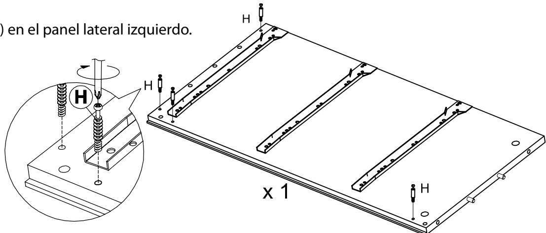
11. Insert 4 cam bolts (H) into the right side panel.
