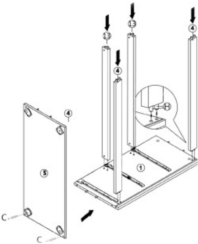
14. With help, align Side panel to assembled rails and bottom. Insert screw (C). Tighten with screwdriver.
