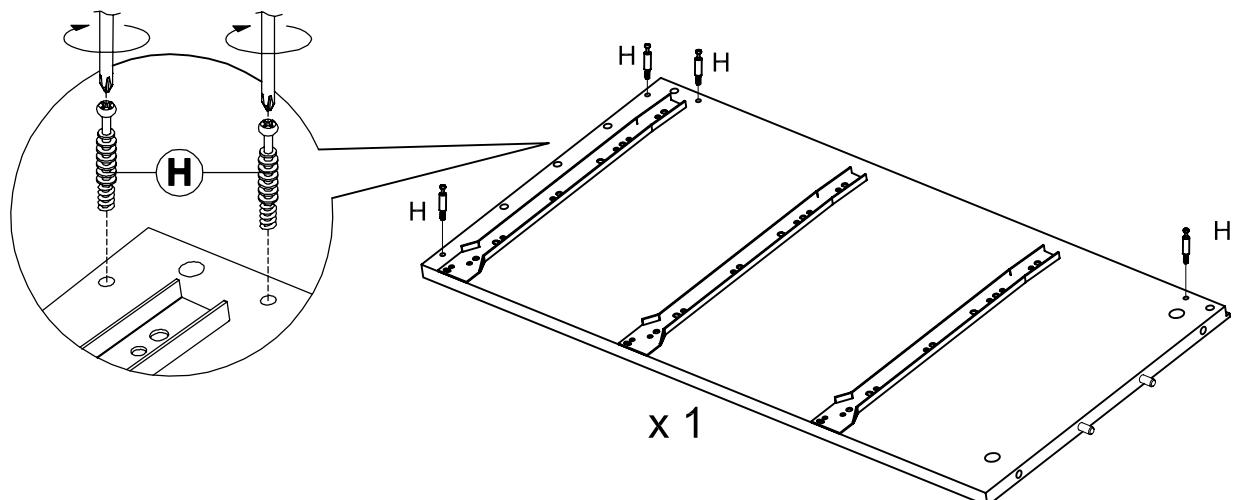
12. Insert 4 cam bolts (H) into the top panel.
