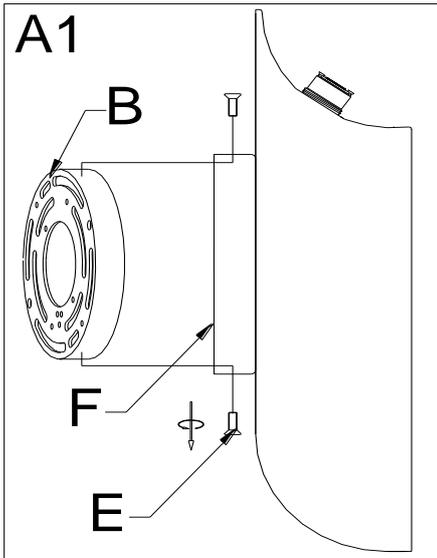
1. Separate the Mounting Plate (B) from the Canopy (F) by removing the Canopy Screws (E). Do not discard the Canopy Screws (E) as these will be used later.
