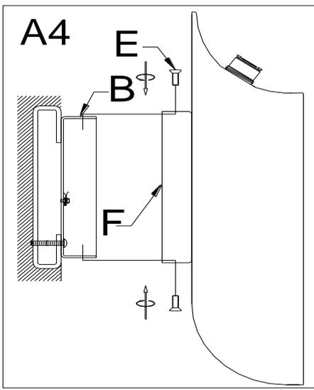
4. Position the Canopy (F) over the Mounting Plate (B), aligning the 2 holes on the Canopy (F) with the 2 holes on the Mounting Plate (B). Secure the Canopy (F) by tightening 2 Canopy Screws (E)
