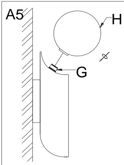
5. Attach the Glass Shade (H) onto the Socket (G) by rotating the Glass Shade (H) in a clockwise direction. Do not over tighten
