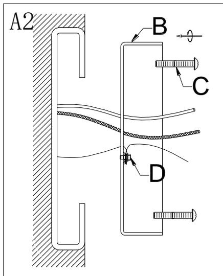
2. Insert the J-box wires through the center opening of Mounting Plate (B). Attach the Mounting Plate (B) onto the wall J-box. Secure the Mounting Plate (B) by turning the 2 Mounting Screws (C) clockwise until tight
