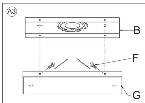
3. Separate the Mounting Plate (B) from the Canopy (G) by removing the 4 Canopy Screws (F). Do not discard the Canopy Screws (F) as these will be used later.
