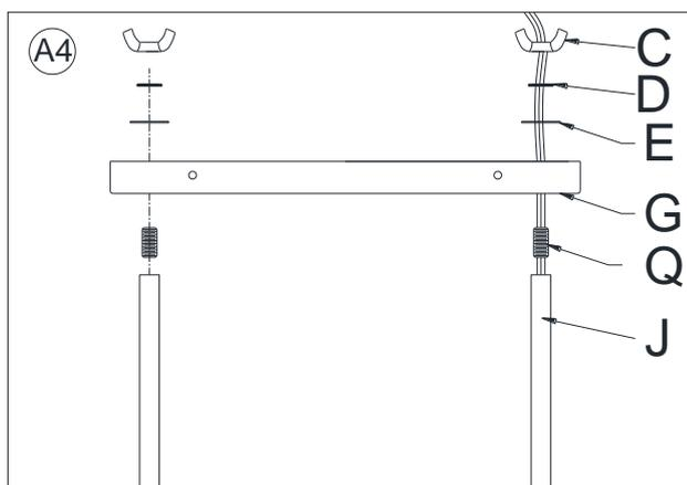
4. Insert the fixture 2 wire power cord and bare copper ground wire through the Nipple (Q) and Canopy (G). Then insert the threaded upper portion of each the long tube (J) into the two holes located near each end of Canopy (G), attach the Metal plates (E) and Key Washers (D) and The Butterfly Nuts (C) onto the thread pipes of the Long Tubes (J) as shown in the diagram. Tighten the Butterfly Nuts (C) by clockwise until tight.
