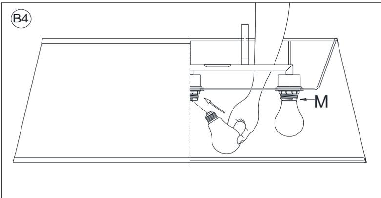
4. Insert the specified light bulbs (Not included) into the Sockets (M). DO NOT EXCEED THE SPECIFIED WATTAGE.
