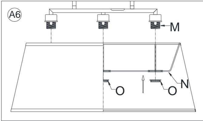
6. Position the Sockets (M) into the Shade Frame (N), secure the Sockets (M) by the Socket Rings (O).
