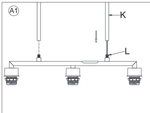
1. Insert the fixture 2 wire power cord and bare copper ground wire through one of the Short Tube (K), and attach bottom end of the Short Tube (K) onto the Threaded Pipe (L) by turning clockwise until tight. Attach another Short Tube(K) onto the other Threaded Pipe (L).
