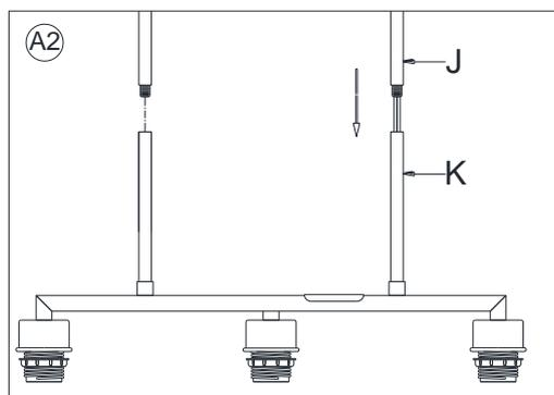
2. Take out 4 Long Tubes (J) from poly bag. If you would like use only a pair of Long Tubes (J), Then thread the 2 wire power cord and bare copper ground wire through the one of Long Tubes (J), Attach the Long Tube (J) onto the top of Short Tube (K) and rotate Long Tube (J) clockwise until tight. Use the additional the Long Tubes (J) as needed to adjust the fixture's suspension length by following the similar
