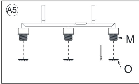
5. Unscrew the Socket Rings (O) from the Sockets (M).
