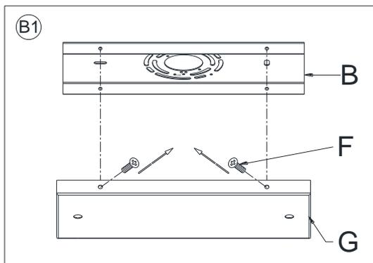
1. Separate the Mounting Plate (B) from the Canopy (G) by removing the 4 Canopy Screws (F). Do not discard the Canopy Screws (F) as these will be used later.
