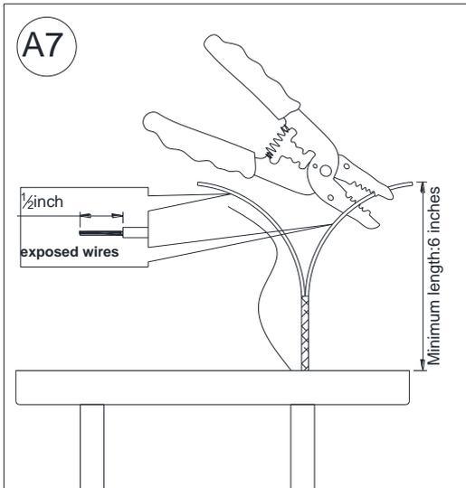
7. If needed, cut off the extra power cord length so that they all are at least 6 inches (152.4 mm) long within the outlet junction box (J-box).
