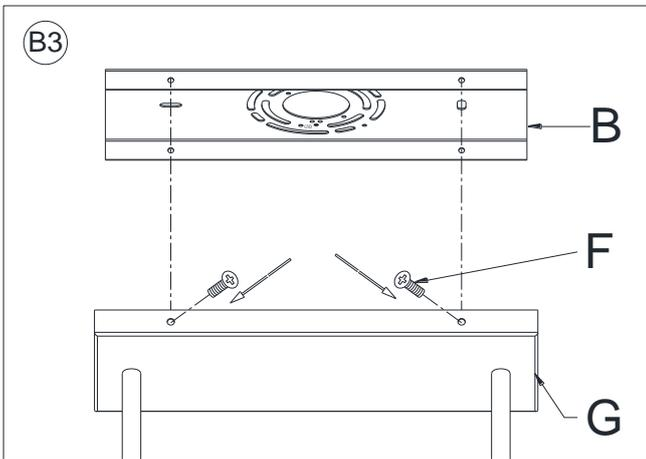
3. With the help of another person to hold the weight of the Chandelier, Raise the Canopy (G) up over the Mounting Plate (B), aligning the 4 holes from the Mounting Plate (B) with the 4 holes on sides of the Canopy (G). Insert the 4 Canopy Screws (F) and tighten each screw with a screwdriver until secure.
