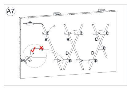
7. Insert the bottom female plug ends of Fixture Rods (D) onto the top male plug ends of Fixture Rods (A/ B/ C) with cross connections as shown. Use the Allen Wrench (C) to tighten the Set Screws (F) (the lower ones, see the enlarged view of the diagram) on the bottom ends of Fixture Rods (D) to secure it in place.
