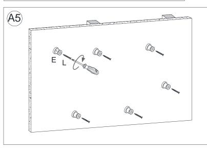
5. Put one Wall Bracket (E) against the wall aligning with installed wall anchor or wall stud. Use the Phillips screwdriver to secure the Mounting Screw (L) through the Wall Bracket (E) and rotate into the wall anchor/stud. Repeat above until all Wall Brackets (E) are secured on the wall. Before tightening the mounting screws, use a tape measure to confirm again the distances between the wall brackets.
