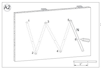
Mark the 6<sup>th</sup> insertion point on the wall through the middle hole of the Steel Template (N) that is 6" spaced from the 5<sup>th</sup> point.
