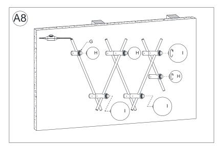
8. Attach the Large Glass Shades (I) and Small Glass Shades (H) onto each Socket (G) by rotating clockwise. The sockets are all in the same size, so you can attach either Large Glass Shade (I) or Small Glass Shade (H) onto any position of these sockets as you wished.
