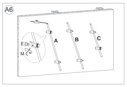
6. Attach the Fixture Rod (A/ B/ C) onto each two Wall Brackets (E) as shown. Use the Allen Wrench (M) to tighten the Set Screws (F) on the bottoms of each fixture rod by rotating in a clockwise direction to secure the Fixture Rods on the wall.
