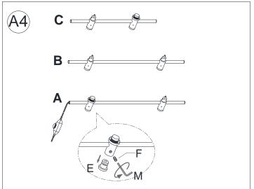
4. Use the Allen Wrench (M) to loosen the Set Screws (F) that located on the bottom of each Fixture Rod A/ B/ C, and then take out the Wall Brackets (E). Don't unscrew Set Screws (F) completely.
