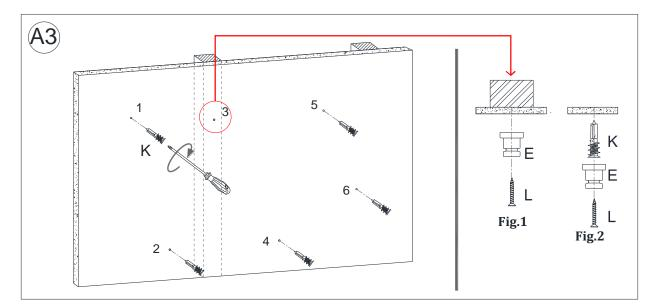
3. First, use a stud-finder to determine if any of the insertion marks aligns to wall stud. If the mark aligns with stud, only use provided Mounting Screw (L) to secure the Wall Bracket (E), see Fig 1. If there is no stud, the Wall Anchor (K) and Mounting Screw (L) are both required, see Fig 2.
