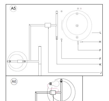
Remove the Threaded Nut (H) and Washer (F) from the Large Glass Threaded (K) and place the 1 pc Washer (F) on to the Large Glass Threaded (K) Attach the Large Glass Shade (L) Please follow the direction of Upward Label to install Glass Shade(L) and place another Washer (F) on to the top of the Large Glass Threaded (K) by tightening the Threaded Nut (H) in a clockwise direction until tight. Removed Label after Installed.
