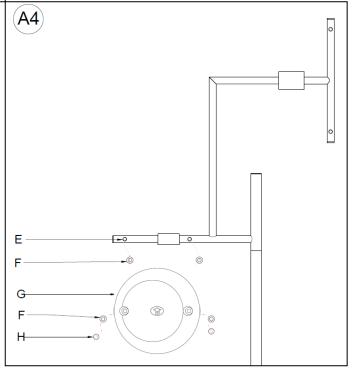
Remove the Threaded Nut (H) and Washer (F) from the Small Glass Threaded (E) and place the 1 pc Washer (F) on to the Small Glass Threaded (E) Attach the Small Glass Shade (G) Please follow the direction of Upward Label to install glass Shade(G) and place another Washer (F) on to the top of the Small Glass Threaded (E) by tightening the Threaded Nut (H) in a clockwise direction until tight. Removed Label after Installed.
