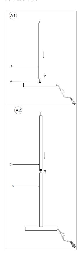
With the help of another person, secure the bottom end of the Lower Stem (B) onto the Threaded Pipe (A) clockwise direction until tight.
