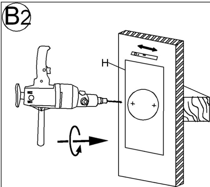
2. Pre-drill pilot holes at the marked locations. This will make installing the Wall Screws (B) onto the wall easier.
