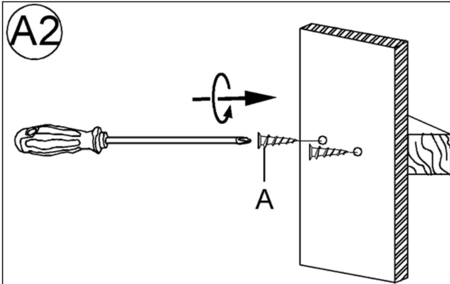
2. Use a Phillips Screwdriver to insert the Wall Anchors (A) at the marked keyhole locations. Do not "push" or drive the Wall Anchors (A) into the wall, it is designed to bore into the wall like a drill bit. Slowly turn the Wall Anchors (A) clockwise while applying pressure until the flange just touches the wall.
