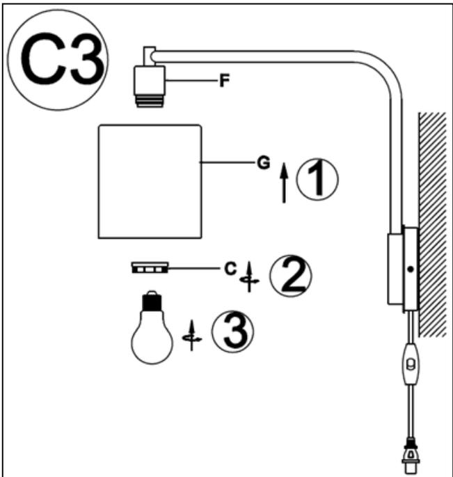
3. Place the Lamp Shade (G) onto the Socket (F). Secure the Lamp Shade (G) by turning the Socket Ring (C) onto the Socket (J) in a clockwise direction until tight. Insert the specified light bulb into the Socket (F). **DO NOT EXCEED THE SPECIFIED WATTAGE.**
