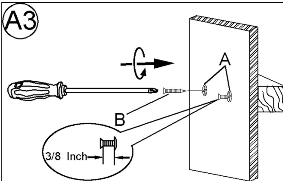
3. Use the Phillips screwdriver to secure the Wall Screw (B) into each installed Wall Anchor (A). Rotate the Wall Screw (B) clockwise until the screw head is about 3/8 inches from the wall.
