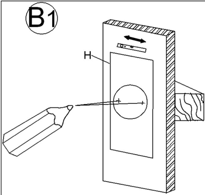
1. Place the Paper Template (H) against the wall at the desired hanging location. Mark the mounting location of the 2 holes of Paper Template (H) onto the wall using a pencil. Use a carpenter's level to ensure a level installation. **MAKE SURE THAT A POWER OUTLET IS REACHABLE BY THE CORD** without straining the cord.
