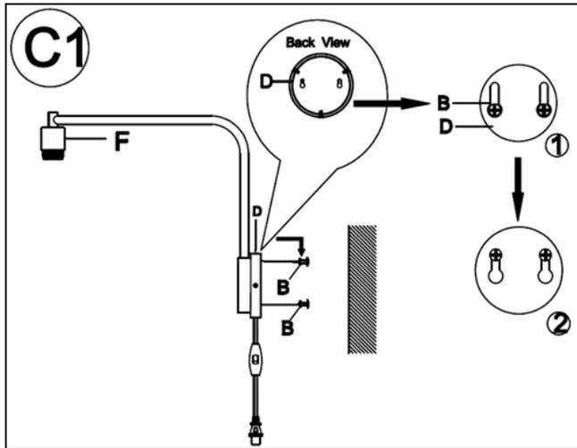
1. Preferably with the help of another person, lift the lighting fixture against the wall so the two mounting keyholes on the Mounting Plate (C) align with and engage the protruding screw heads (B). Gently lower the lighting fixture so that the screws support its full weight. Make sure that each screw (B) is completely engaged with its keyhole before releasing the fixture.
