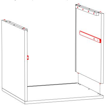
11: To completely secure bottom panel, insert long connecting screws (K) into holes provided on bottom panel.
