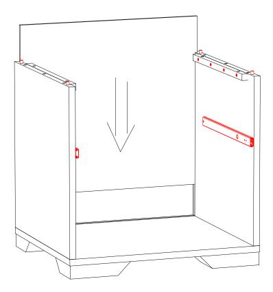
14: Attach top panel to dowels in upper edge side panels. Insert short connecting screws (H) in holes provided.
