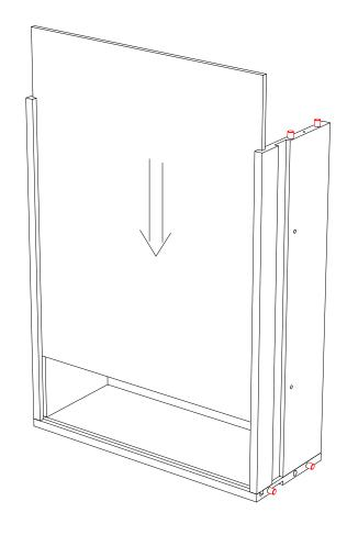
5: Insert 4 screws (D) into holes provided on drawer sides to complete assembly of drawer box.
