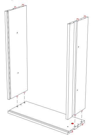
4: Attach left drawer side panel to drawer front and back panels using factory installed dowels.
