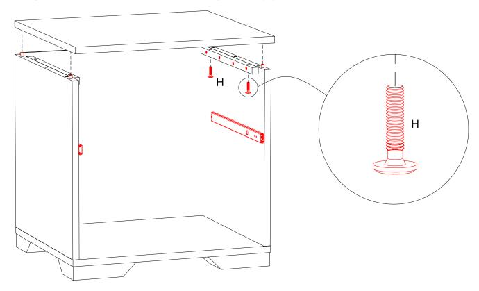
15: Slide the drawer onto drawer rails. Insert connecting screws (I) into holes provided inside drawer side panels.
