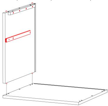
10: Attach right side panel into holes provided in bottom panel.
