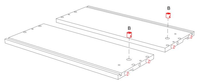
2: Attach drawer front and back panels to right drawer side panel using factory installed dowels.
