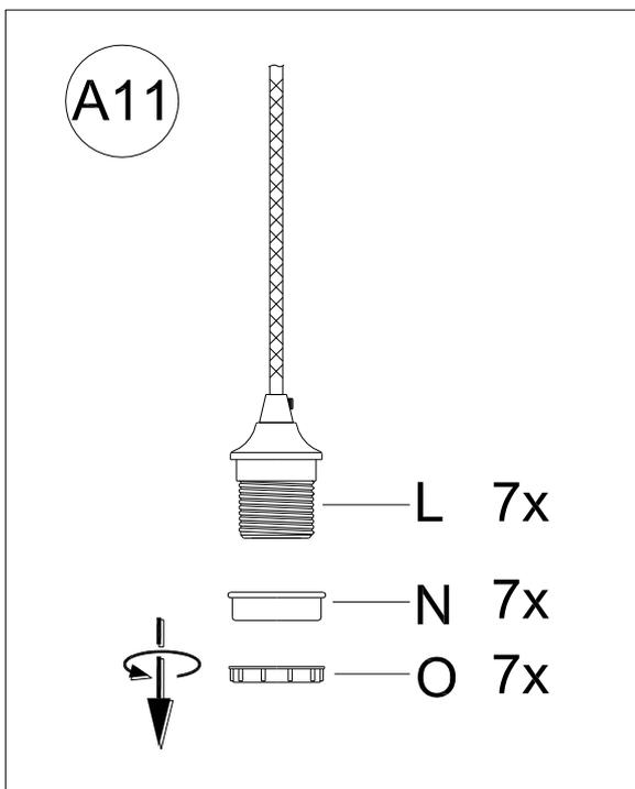
Unscrew each Socket Ring (O) from each Socket (L) and remove Metal each **Spacers** (N).
