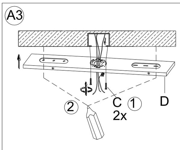
1. Determine the desired location of the light fixture and temporarily install the Mounting Plate (D) to the ceiling outlet box using the 2 J-box Mounting Screws (C), insert and tighten each screw until the Mounting Plate (D) is firmly secured to the J-Box.
