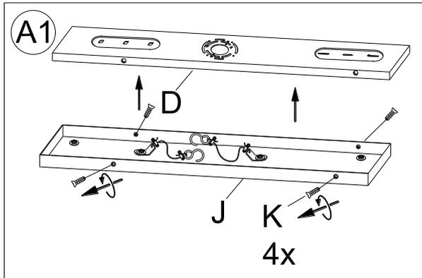
Separate the Mounting Plate (D) from the Canopy (J) by removing the 4 Canopy Screws (K). Do not discard the Canopy Screws (K) as these will be used later.
