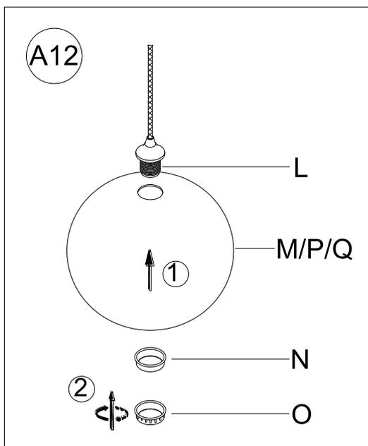
1. **Raise one Large Glass Shade (M) over one of Sockets (L), while holding the Large Glass Shade (M) in place, place one Metal Spacer (N) over the Socket (L) and tighten the Socket Ring (O) in a clockwise direction by hand until tight.**
