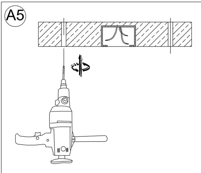
Using the drill with the appropriate size drill bit (just large enough to make hole that will allow passage of the folded Toggle Wings (F) of the Toggle Bolts (E)), drill 1 hole in the ceiling at each of the 2 marked slot locations for the toggle bolt and Toggle Wings assemblies.
