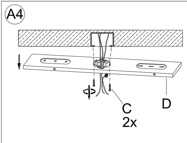
Un-installing the Mounting Plate (D) from the marked ceiling outlet box location by loosening and removing the 2 J-box Mounting Screws (C) with a screwdriver.
