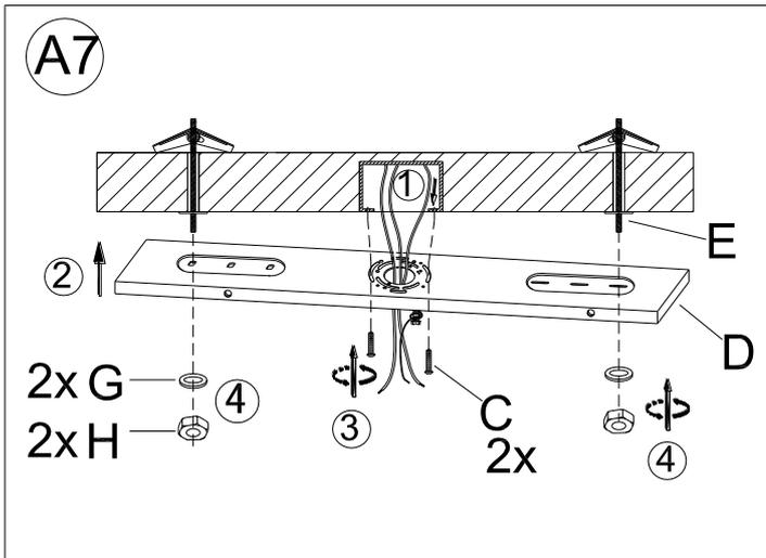
1. Gently pull the existing wire down from the ceiling junction box and allow wires to hang through the center opening of Mounting Plate (D).
