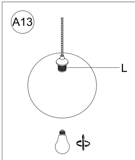
Insert the specified light bulbs into the Sockets (L). DO NOT EXCEED THE SPECIFIED WATTAGE.
