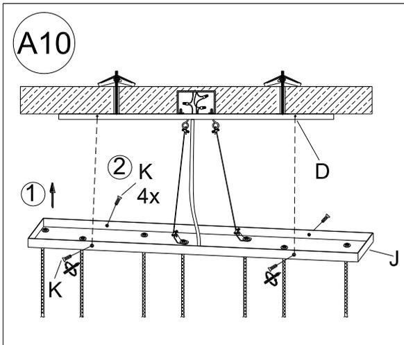
1. Raise Canopy (J) up over the Mounting Plate (D), align the holes in the Mounting Plate (D) with the holes on the side of the Canopy (J).
