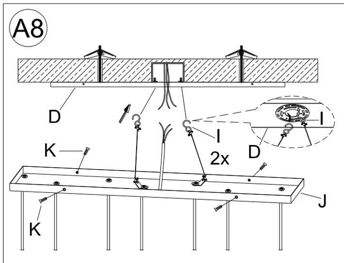
With the help of another person to hold the weight of the **chandelier**, securely attach the “S” Hooks (I) of each safety cable onto the slots of Mounting Plate (D). Now the chandelier can be supported by these 2 safety cables.
