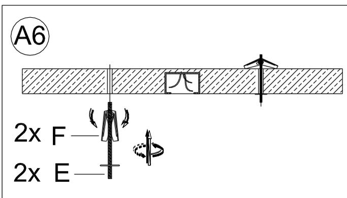
Use the **assembled** Toggle Bolts and Toggle Wings (E&F), inserted through each of the 2 ceiling holes, making sure only the Toggle Wings (F) are fully inserted into the ceiling and Toggle Wings (F) are open. Rotate each Toggle Bolt (E) in a clockwise direction until its flat washers on the Toggle Bolts (E) tight against the ceiling.
