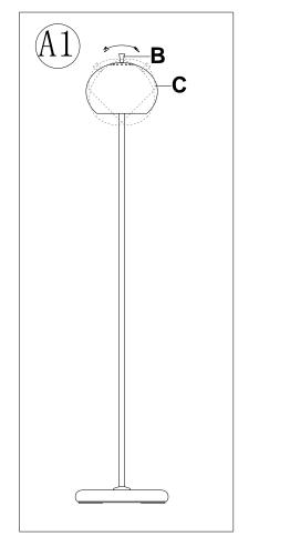
1. If needed, adjust the Metal Shade (C) to the desired position at 0° to 90° by Shade Handle (B).
