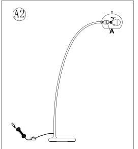
Insert the specified light Bulb into the Socket (A). DO NOT EXCEED THE SPECIFIED WATTAGE.
