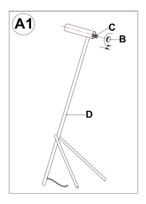
Unscrew the Thumb Screw (B) from the Threaded Nipple (C) of the Lamp Body(D).
