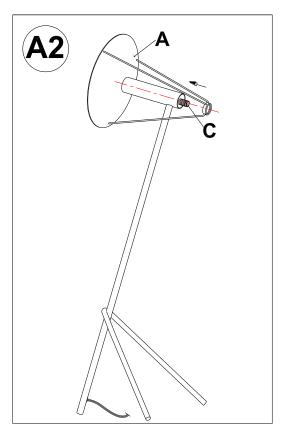
2. Place the Diffuser (A) onto the Threaded Nipple (C).
