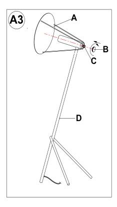
3. Secure the Diffuser (A) by tightening the Thumb Screw (B) in a clockwise direction.
