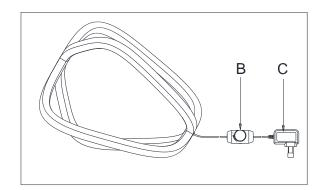
Insert the Plug into the socket. Rotate the Switch (B) to turn on the light.
