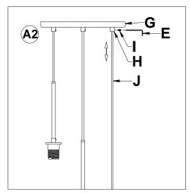
2. Loosen the Set Screws (I) from the Holder Tubing (H) under the Canopy (J) using a Allen Wrench (E) by turning counter-clockwise. Adjust the Power Cord (J) upwards or downwards through the Canopy (G) until a new desired suspension length is determined. Secure the Power Cord (J) in place by tightening the Set Screws (I) onto the Collars (H). Do not over tighten the screw, making sure the Power Cord (J) will not slip downwards with the pendant body.
