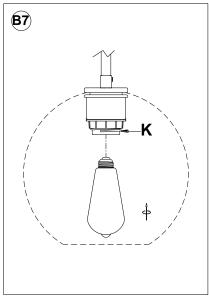
7. Insert the specified light bulb into the Sockets (K). DO NOT EXCEED THE SPECIFIED WATTAGE.
