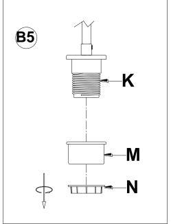
5. Unscrew the Socket Rings (N) and Spacers (M) from the Sockets (K).
