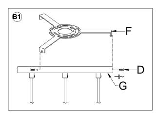
1. Separate the Mounting Plate (F) from the Canopy (E) by removing the 3 Canopy Screws (D). Do not discard the Canopy Screws (D) as these will be used later.
