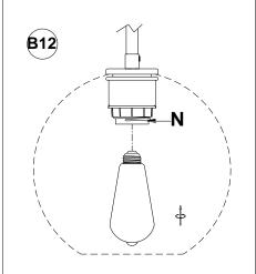
12. Insert the specified light bulbs into the Sockets (N). DO NOT EXCEED THE SPECIFIED WATTAGE.
