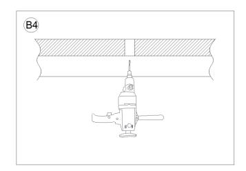
Using the drill with the appropriate size drill bit (just large enough to mark hole that will allow passage of the folded Toggle wrings(E) of Toggle Bolts(F), Drill 1 hole in ceiling at each of the 2marked slot locations for the Toggle Bolts (F) and Toggle Wings (E) assemblies
