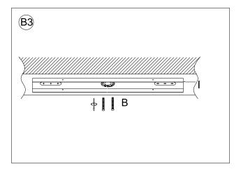
Un-install the Mounting Plate (I) from the marked ceiling outlet box location by loosening and removing the two Mounting Screws (B) with a screwdriver.
