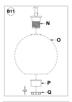
Put the Glass Shades (O) (Packed separated) and Spacers (P) onto the Sockets (N), secure Glass Shades (O) (Packed separated) and Spacers (P) by rotating the Socket Rings (Q) in a clockwise direction until tight.
