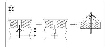
5. Use the assembled Toggle Bolts and Toggle Wings (F&E), inserted through each of the 2 ceiling holes, making sure only the Toggle Wings (E) are fully inserted into the ceiling and Toggle Wings (E) are open. Rotate each Toggle Bolt (F) clockwise until each flat washer on the Toggle Bolt (F) is tight against the ceiling.
