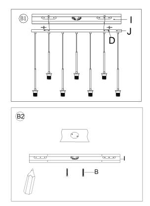
Separate the Mounting Plate (I) from the Canopy (J) by removing the 4 Canopy Screws (D). Do not discard the Canopy Screws (D) as these will be used later.
