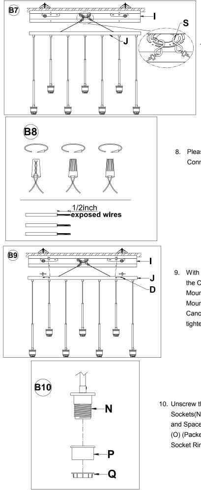
With the help of another person to hold the weight of the Chandelier, Raise the Canopy (J) up over the Mounting Plate(I), Attached the Hooks(S) to the Mounting Plate (I).
