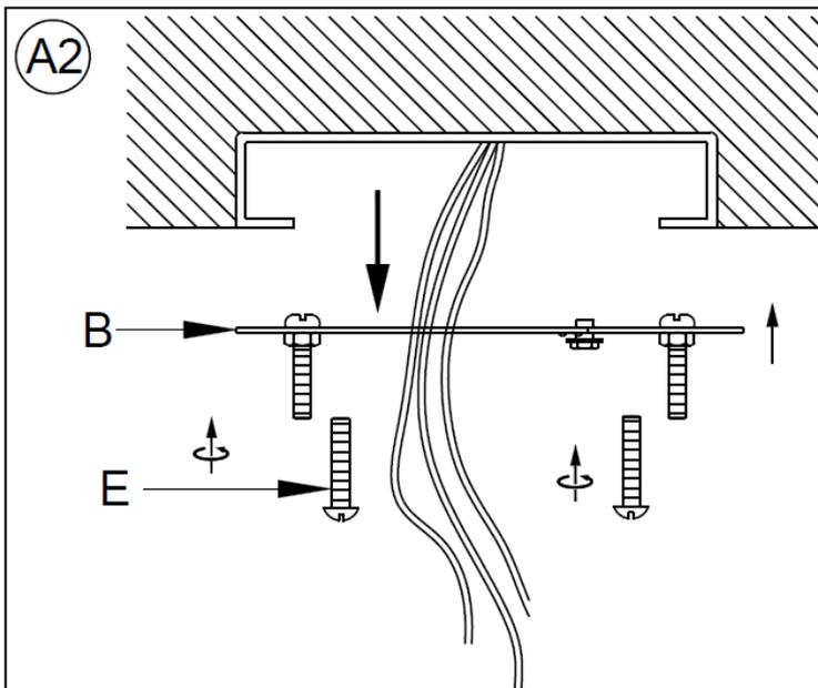
1. Insert the J-box wires through the center opening of the Mounting Plate (B)
