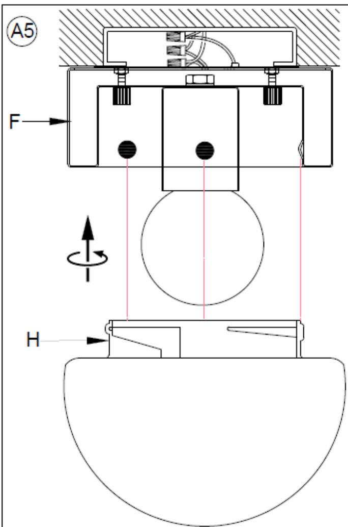
Insert the Shade (H) opening into the Canopy (F) aligning 3 protrusions from inner of the Canopy (F) with the threaded channel on the Shade (H) and rotate the Shade (H) in clockwise direction until the protrusions are tightly wedged against the threaded channel.
