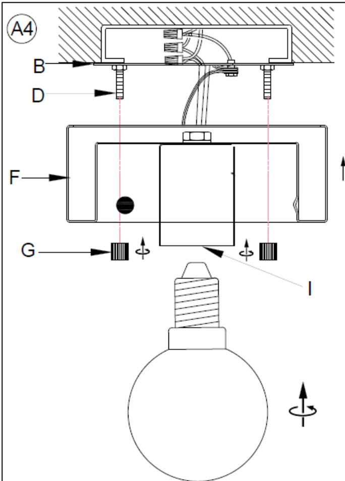
1. Position the Canopy (F) over the Mounting Plate (B), making sure the 2 Threaded Rods (D) extend through the 2 holes on the Canopy (F). Secure the Canopy (F) by turning the Knurled Nuts (G) onto the exposed threaded portion of Threaded Rods (D) clockwise until tight.
