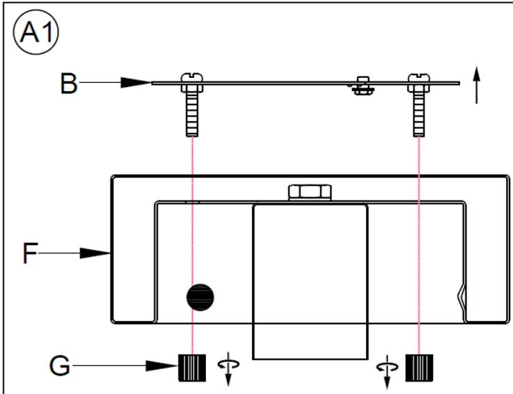
Separate the Mounting Plate (B) from the Canopy (F) by removing the 2 Knurled Nuts (G).
