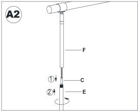
Insert the Male Plug (C) through the Bottom Tube (E). And attach the top end of Bottom Tube (E) onto the bottom end of Top Tube (F). Turn the Bottom Tube (E) in a clockwise direction until tight.
