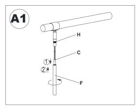
1. Insert the Male Plug (C) through the Top Tube (F). And attach the Top Tube (F) onto the Threaded Nipple (H) by turning the tube in a clockwise direction until tight.
