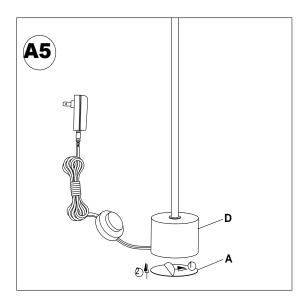
5. Peel off paper cover on the Pad (A), and Stick the Pad (A) at the bottom of the Metal Base (D)
