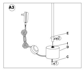
Insert the Male Plug (C) through the Metal Base (D). With the help of another person, place the bottom end of the bottom tube (E) onto the Threaded Pipe (I) of the Lamp Base (D) and rotate the base in a clockwise direction until tight.
