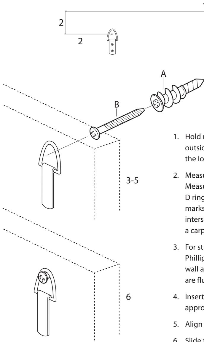
! For drywall mounting, use anchors with screws.
