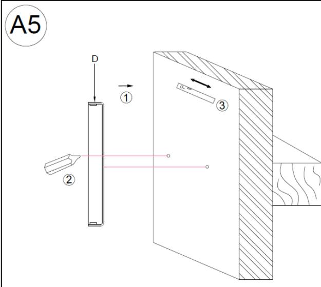
1. Place the Mounting Plate (D) against the wall at the desired hanging location.
