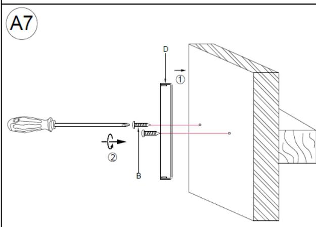
1. Attach the Mounting Plate (D) onto the wall aligning the 2 slots on Mounting Plate (D) with the 2 marked locations.
