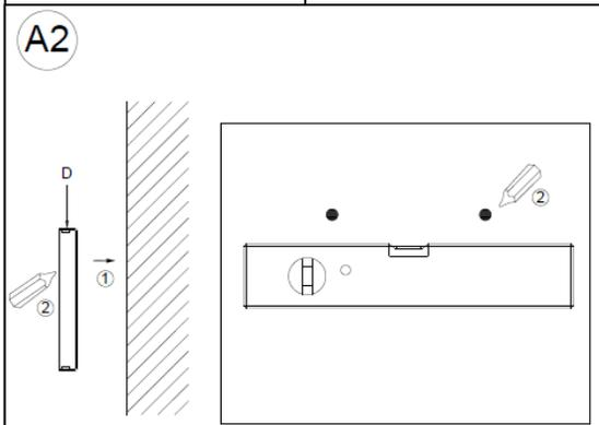
1. Place the Mounting Plate (D) against the wall at the desired hanging location.
