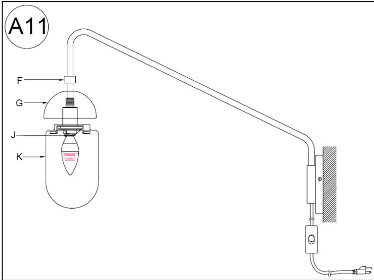
1. Lower the Metal Cap (G) until the edge of the Metal Cap (G) is fully contacted and aligned with the upper outer edge of the Glass Shade (K). Secure the Glass Shade (K) by turning the Threaded Nut (F) onto the threaded portion at the top of the Socket (J) in a clockwise direction by hand until tight. Do not over tighten.
