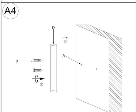
1. Attach the Mounting Plate (D) onto the wall aligning the 2 slots on Mounting Plate (D) with the 2 installed Wall Anchors (A).
