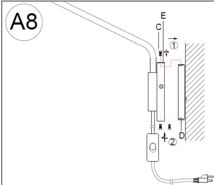
1. Place the Canopy (E) onto the installed Mounting (D) aligning the holes on the top and bottom of the Canopy (E).
