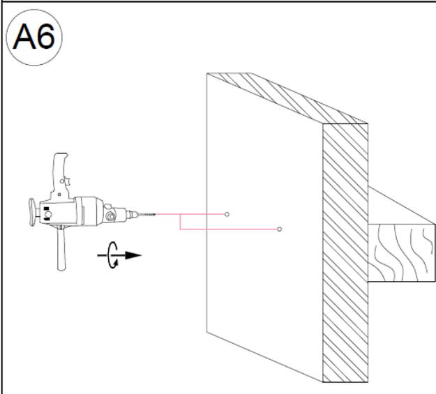
1. Pre-drill pilot holes at the marker locations. This will make installing the Wall Screws (B) onto the wall easier.
