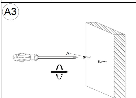
1. Use a Phillips Screwdriver to insert the Wall Anchors (A) at the marked keyhole locations. Do not "push" or drive the Wall Anchors (A) into the wall, it is designed to bore into the wall like a drill bit. Slowly turn the Wall Anchors (A) clockwise while applying pressure until the flange just touches the wall.
