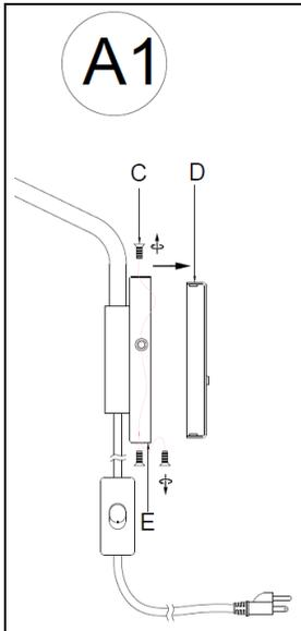
1. Separate the Mounting Plate (D) from the Canopy (E) by removing the 3 Canopy Screws (C). Do not discard the Canopy Screws (C) as these will be used later.
