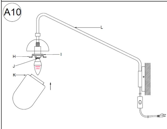
1. Position the Glass Shade (K) over the Metal Plate (I) by inserting the Socket (J) and Metal Plate (I) into the opening of the Glass Shade (K) in a slanted direction until the 2 Plastic Pads (H) on the Metal Plate (I) are contacted and engaged with the interior shoulder surface of Glass Shade (K)
