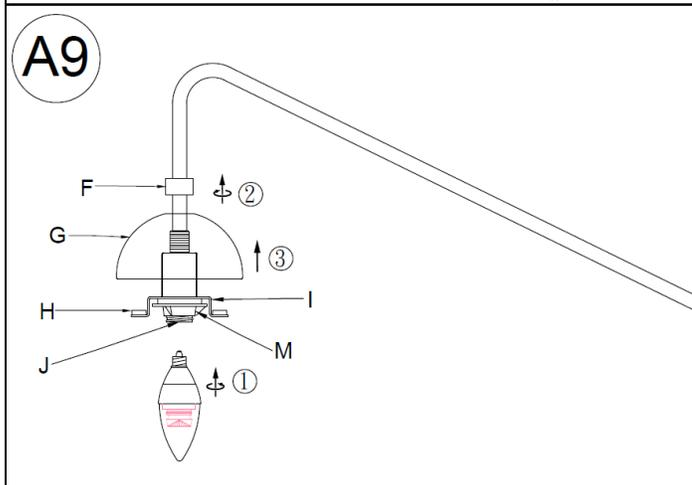
1. Insert the specified light bulb into the Socket (J) **DO NOT EXCEED THE SPECIFIED WATTAGE.**
